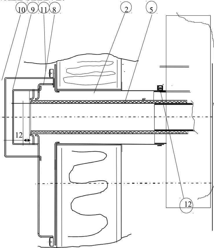
1. Make a  $\varnothing 90$  mm hole to the wall, whose midpoint is at a height of 225 millimetres from the bottom of the heater.
