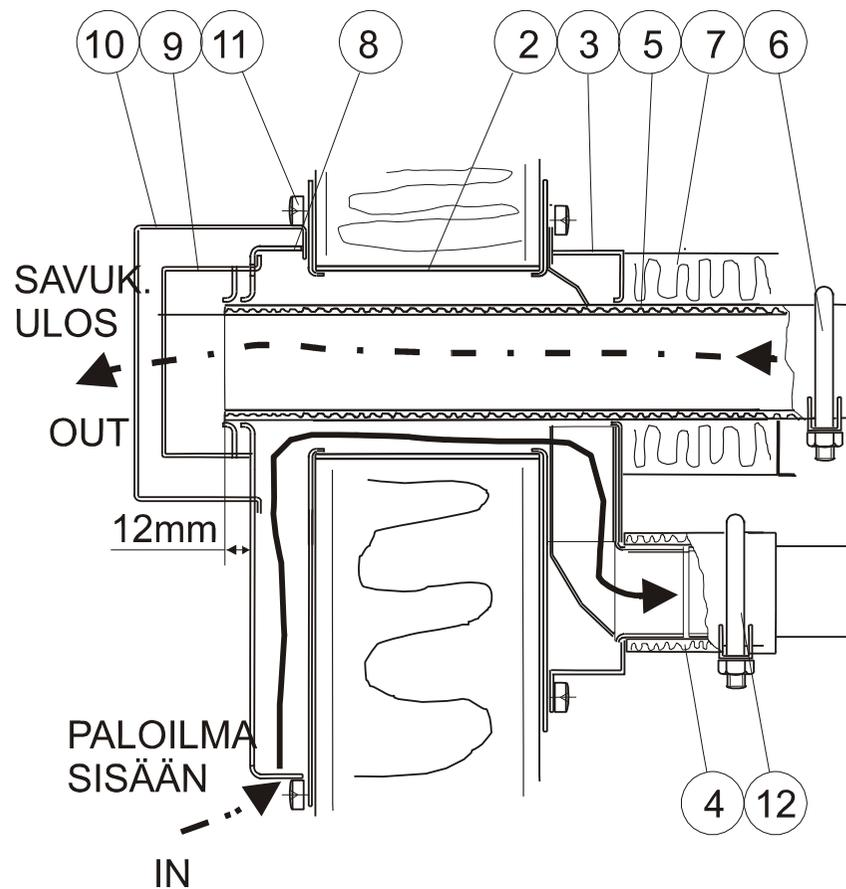
1. Make a  $\varnothing 90$  mm hole to the wall, whose midpoint is at a height of 225 millimetres from the bottom of the heater.
